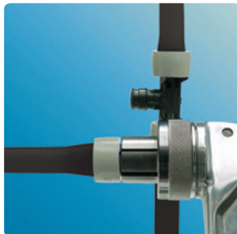
Expanding the pipe end
